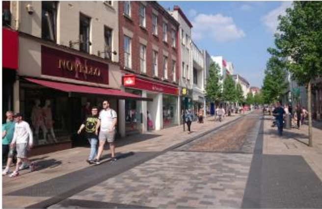
Example of shared space environment with surface treatments indicating zones of use, well-marked informal pedestrian crossings, and pedestrian oriented urban realm
