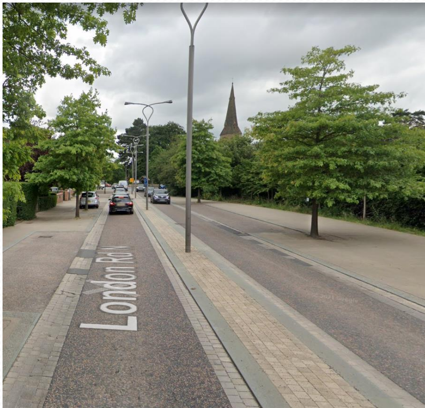
Example of carriageway separation for Option A
