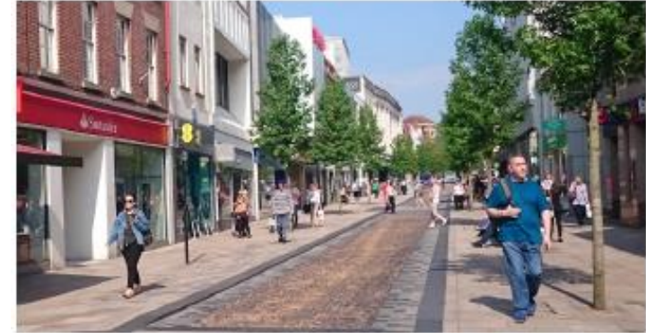
Textured edge bands to visually narrow road space and calm traffic speed
